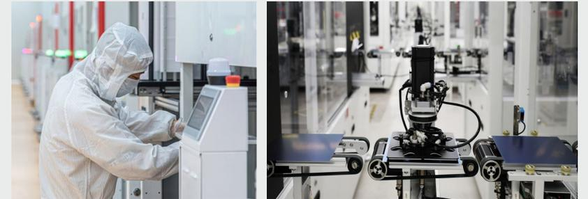
**The module production workshop:** adopt intelligent production line and automatic optical inspection and judgment equipment (based on AI technology) to detect the defects of module products visually and replace the traditional manual detection, enhancing the test efficiency and improving product yield. Intelligent production line equipment has adopted precise positioning welding solutions and achieved millimeter-level precision positioning required for MBB module production.
