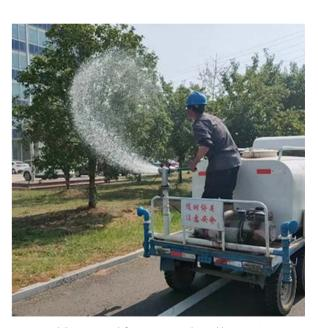
Mobile water truck for greening and sprinkler irrigation
